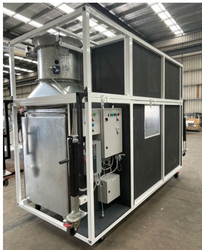
AMCA's purpose-built training pods (such as the stair pressurisation pod above) are fitted with the latest equipment, enabling students to be trained and assessed in a simulated work environment.
